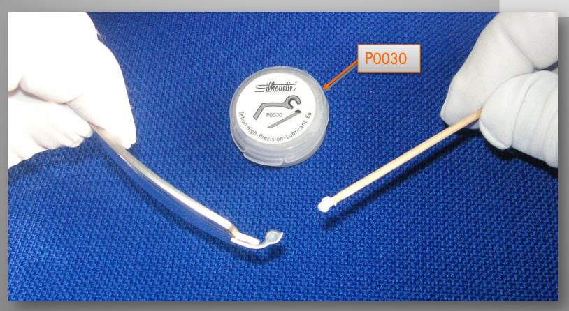
Grease inside loop of hinge with high precision lubricant teflon. If neccessary clean beforehand. Attach plastic plate and mount temple.
