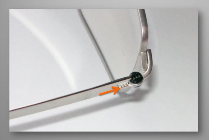
Place temple exactly at the slot of the BLS-hinge and click it in carefully until it stops.
