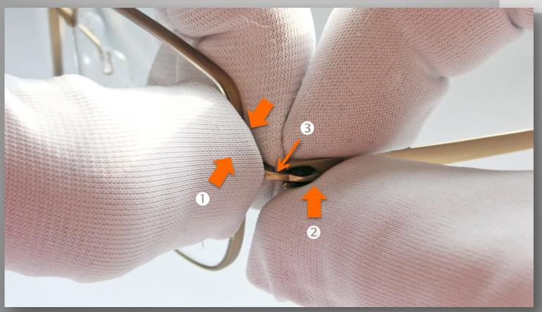
Hold side part firmly at frame eye rim. Cover temple edge with hinge closely. Adjust inclination at Titanium part.
